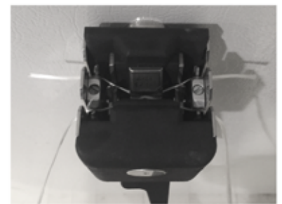
ends opposed splicing with special yarn clamps for delicate fibers
